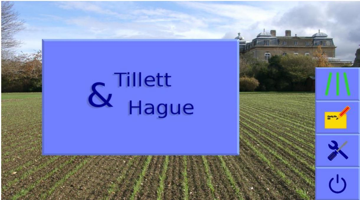
From this screen you have the option to enter the Inter-row working screen (Three green crop rows symbol), Service Tools Menu (Spanner and screwdriver symbol) or the Configuration File Editor (Pen and paper symbol). This abbreviated version of the manual only covers the working screen. For more information consult the full reference manual.
