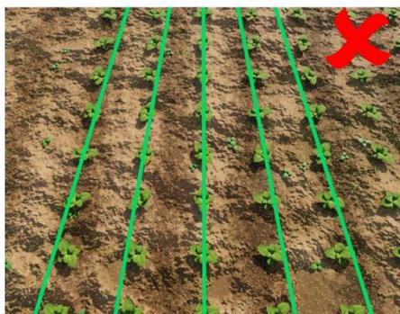
If template lines appear narrower than crop rows at the top of the image but wider at the bottom, rotate the camera up so it views further ahead.
