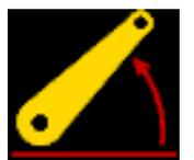
Lifting the implement should result in the "stopped" symbol being replaced by the "lifted" (yellow lift arms) symbol.
