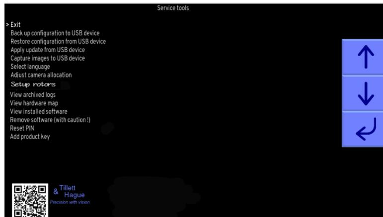
From the start-up screen users can enter a service menu by touching the tools symbol. The service menu, illustrated above, offers a number of tools that can be useful in maintaining or fault finding a system. The QR code defaults to our web site but can be configured as part of branding.
