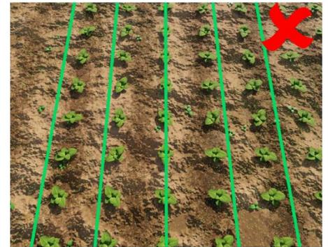
If the template matches mid screen, but not at the top or bottom, check that the implement is level. If it is, camera inclination angle may need adjusting.
